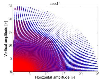
Stable particles (red) among all simulated particles (blu), for one configuration of dipole field errors in the accelerator.
